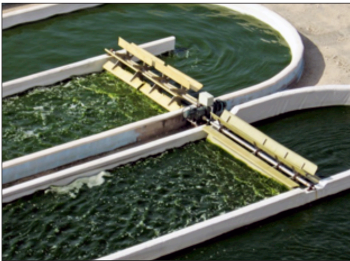
Figure 3. Section of a raceway pond and paddle wheel mixing. Photo courtesy of Nature Beta Technologies LTD, EI.
